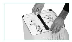
4. Take a firm grip and then pull the hatch upwards.
