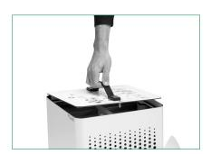
5. Grip the handle on top of the filter and pull it towards you. Put the filter in a plastic bag. Repeat procedure on the other filter and place in a plastic
